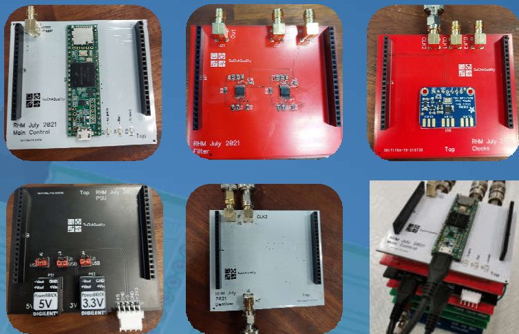
Figure 2. Example boards from the low cost console. Clockwise from top left: Main board, two stage capacitive filter, clock module, completed stack, demixing module and power supply module.
