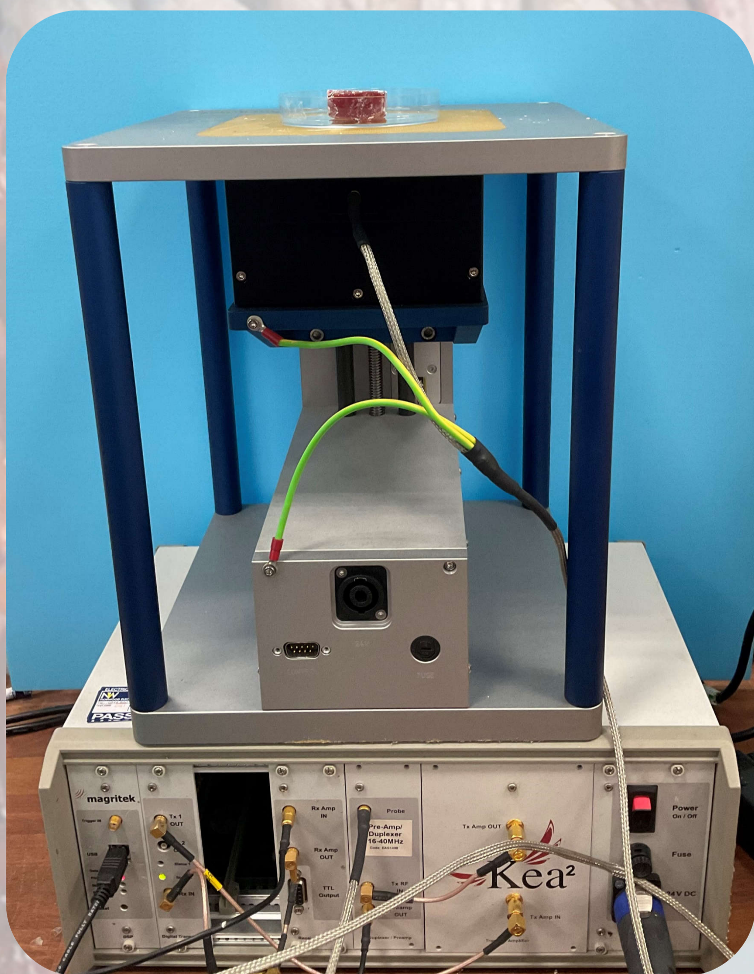
Figure 1 Left - Photograph of a Turkish Delight sample in the scanning position on top of the MR-MOUSE®. Top - Example of Turkish Delight Samples
