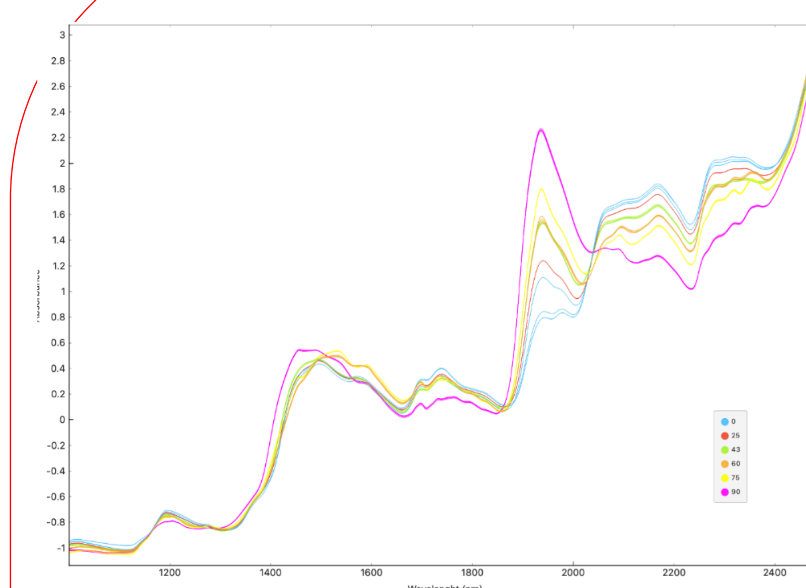
Figure 3: Buchi NIR - fat-free milk powder spectra after Savitsky-Golay (15-2) and SNV preprocessing.
